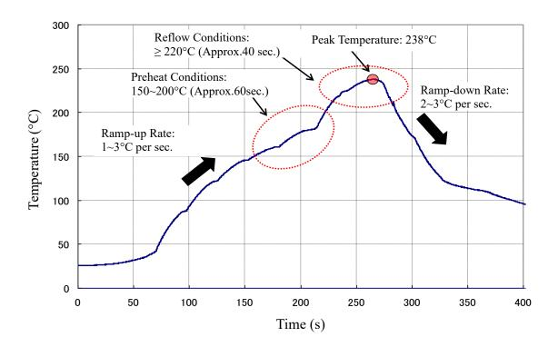
Figure 4. Actual temperature measured profile as target set-up for M705 paste
